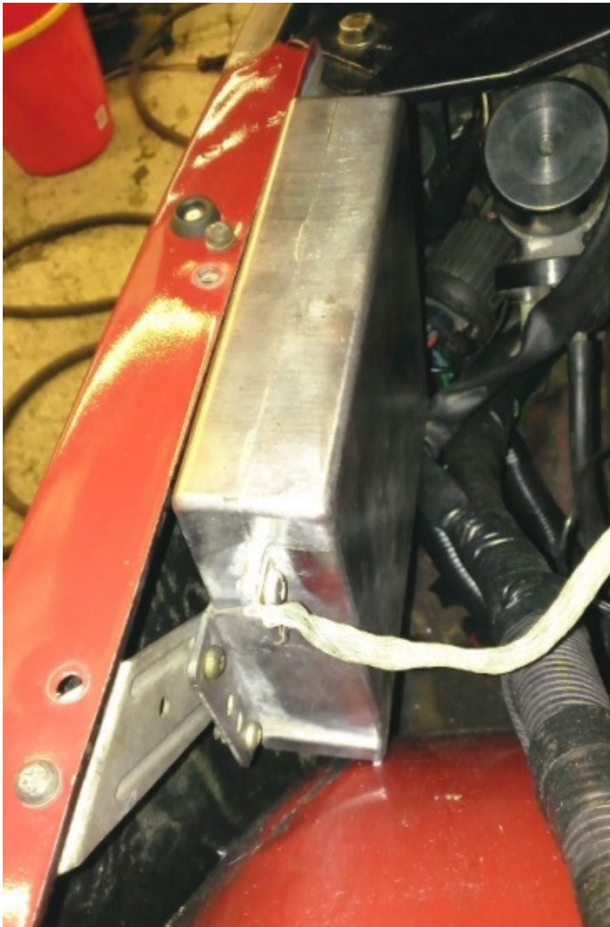
Trionic 5.5 ECU mounted using original 900 APC brackets in the original 900 APC location
